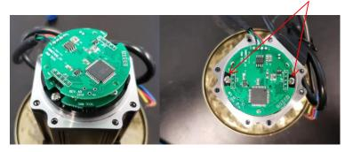
Make sure magnetic hub is not rubbing against encoder PCB. There should be approximately 1.5mm space between the top of magnetic hub and encoder PCB.
