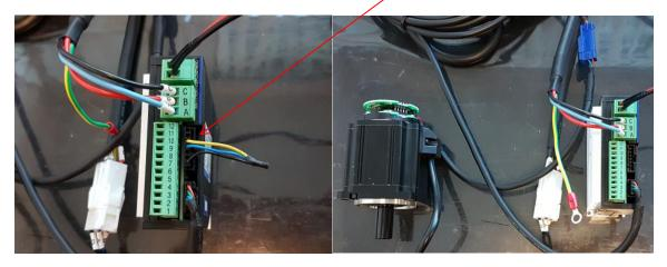
(7) Power ON the servo drive. The motor will rotate **clockwise** for 20~30seconds, then stop – this is the encoder tuning/zeroing procedure. After the motor has stopped, wait 10seconds, then the shaft will become free to indicate that the tuning has completed. Do not touch the motor shaft anytime during the tuning procedure unless it has finished and the shaft is free. Power OFF the servo drive. Proceed with this tuning procedure 3 more times.
