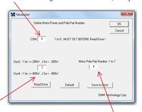
Set the left parameter according to current output. If the motor's peak current draw is less than 10A, set to "1". If the current draw is more than 20A, set to "2".
