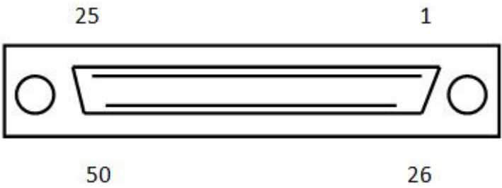
Fig. 109 Description of the ports on the back of the CN1 connector
